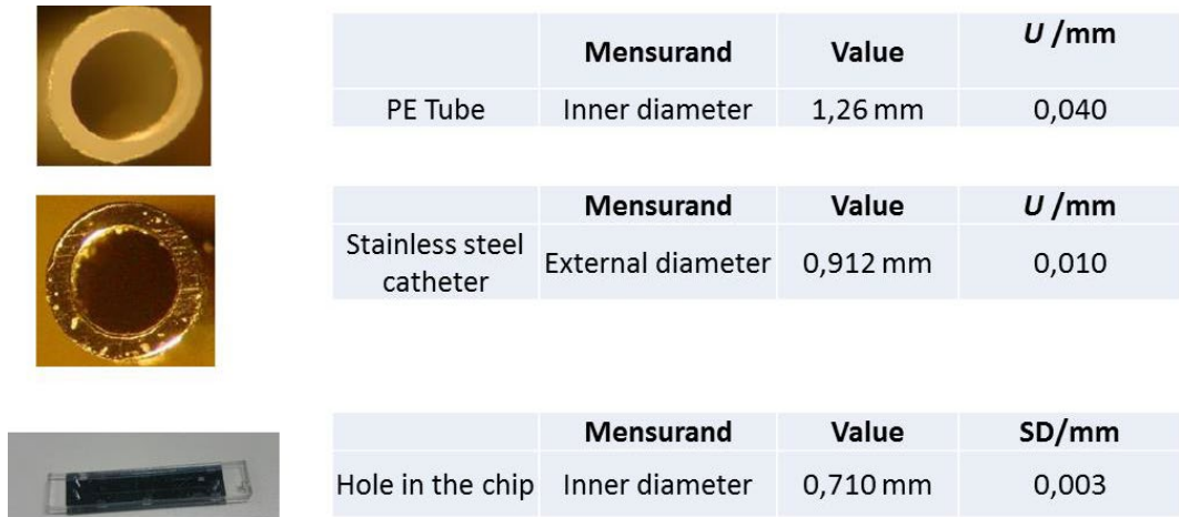
Figure 16. Dimensions measured using the interferometer for the PDMS chip.
